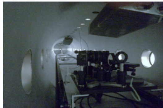
Fig.17: Grazing incidence filament beam profiler on the rail inside CLAPTAM
