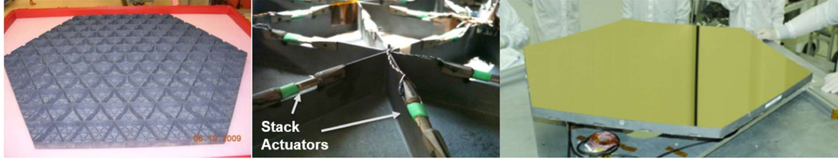
Figure 2. Three views of a SiC mirror for warm VIS applications, showing the as-cast part with its isogrid back structure, ceramic actuators integrated into the isogrid main ribs, and the facesheet.
