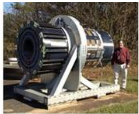
Figure 3: The VETA-II test article for the Chandra X-ray observatory 11 . This "Verification Engineering Test Article" enabled alignment of the main mirror elements and uncovered major design risks.
