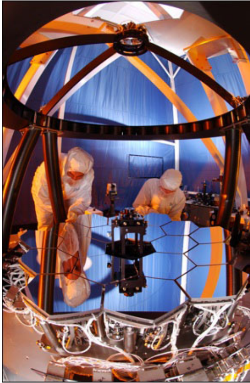
Figure 3: The VETA-II test article for the Chandra X-ray observatory 11 . This "Verification Engineering Test Article" enabled alignment of the main mirror elements and uncovered major design risks.
