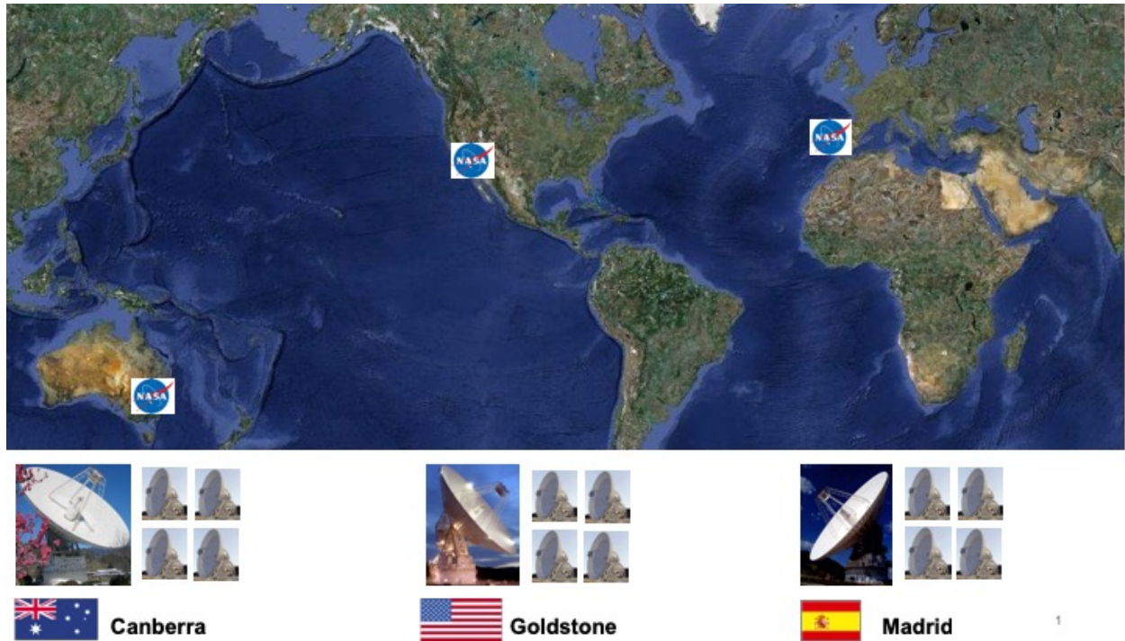
Figure 1. By the middle of the 2020s, NASA's Deep Space Network will have five antennas at each of its three Complexes, one 70 m-diameter antenna and four 34 m-diameter antennas, providing the capability to obtain high data rates ( > 300 Mbps) and large data volumes for Astrophysics missions.
