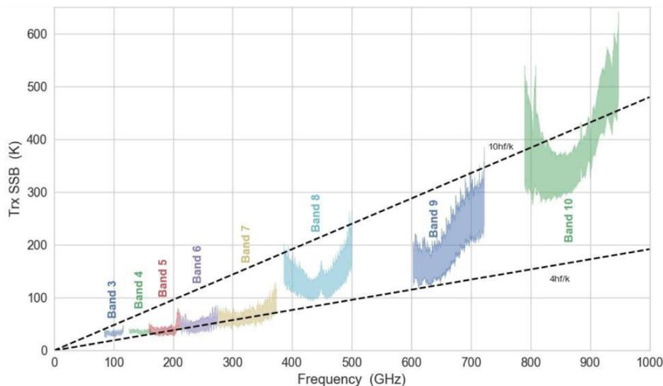
Figure 5: *Current ALMA receiver temperature  $T_{rx}$  (i.e. sensitivity, single sideband) vs. sky frequency, colored by band. The two dashed lines indicate  $4\times$  and  $10\times$  the quantum limit. **Improvements are possible in the bands that have  $T_{rx}$  above the lower line.***
