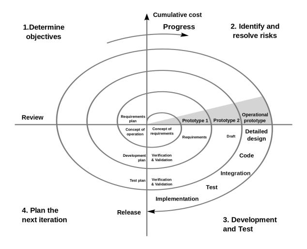
Figure 1. A diagram showing the 4-Steps of Boehm's Spiral Development Model, which also apply to other process models, such as incremental, waterfall, or evolutionary prototyping.
