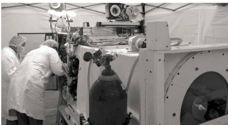
Fig. 14 – The vector spectromagnetograph (VSM) for the NSO SOLIS instrument set. A similar device would be a component of ngGONG.
