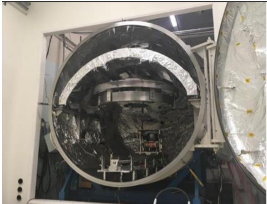
Figure 4 – ZeCoat's 2.4-meter motion-controlled vacuum coating system is large enough to coat segments up to 2-meters in diameter (1.3-meter MCAT primary mirror shown in photo)
